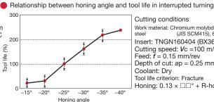
**Cutting conditions** Work material: Chromium molybdenum steel (JIS SCM415), 60 HRC Insert: TNGN160404 (BX360) Cutting speed: Vc =100 m/min Feed: f = 0.15 mm/revDepth of cut: ap = 0.25 mm Coolant: Drv Tool life criterion: Fracture Honing: 0.13 × □□° + R-honing
